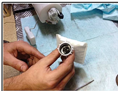
5. Reassemble the valve inside the filter
