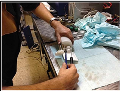
1. Remove the fuel filter
