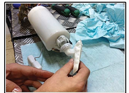
6. Reinstall the fuel filter
