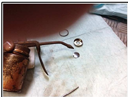
4. Lubricate the valve plate
